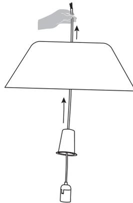
2 Thread the cord through the lampshade from underneath.
