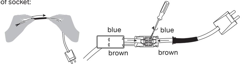
5 Insert the ceiling plug cord through the rubber sleeve.
