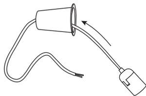
1 Thread the cord through the cone-shaped cup.
