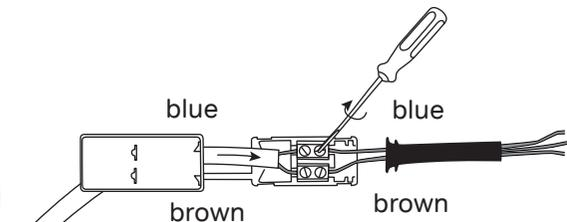
6 Open the screws of two poles terminal block, insert the ends of the cord and the ceiling wires (not the yellowgreen wire) in their places and tighten the screws firmly.
